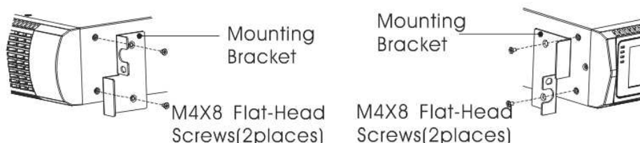
FIG.5 Installation des supports de montage
