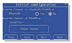
In dialogue 2, you can choose the inverter manufacturer, that is attached via the RS485-A interface. Note that the MT Sensor Box is also treated like an inverter and therefore runs as type "MT Sensor".
