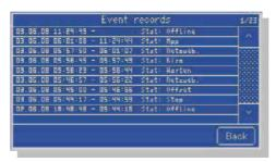
The event log records all status changes to the inverter in a separate protocol. Every 15 seconds (depending on the number and type of the inverter sometimes even longer), the status and error codes are read from the inverters. If there's a change, it gets saved in the log. Every inverter has 200 memory slots available. The current status is always at the very top of the list in dialogue Page 1.
