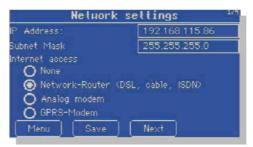
Here you can configure the IP address and subnet mask. The factory default address is 192.168.178.49 and needs to be adapted so that access via a PC is possible. Then you define the appropriate internet access for you.
