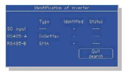
Every interface is shown with the predefined inverter-type, and everything is examined in turn. This process can be relatively long, such as when Sputnik/SolarMax searches through a 253 address range.
