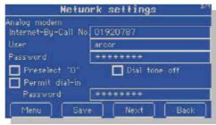
If a telephone line is available, the SoleilLog<sup>1000</sup> can with the help of the SoleilLog<sup>1000</sup> Modem Package gain access to the Internet. This is always necessary when you want to receive information remotely per email, SMS or on the homepage.
