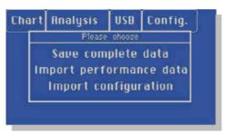
The data backup can be done any time onto a USB stick or back to the USB stick. All data is saved (Day curves max. 60 days), i.e. the configuration and measurement data. When restoring the data, the measurement data or the configuration can be selected individually.
