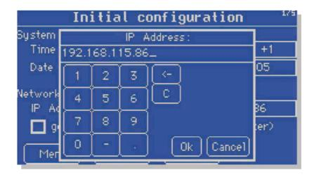
The virtual keyboard if needed appears on the display and you can carry out appropriate entries just like a normal keyboard. Depending on the type of entry, a numeric keypad or a full alphanumeric keyboard will be shown.
