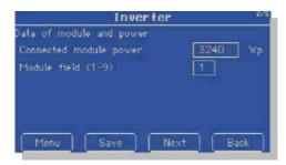
• Module field Via the "Module field", the same strings for system monitoring are merged together and monitored together. For a roof with the same modules, same orientation and identical roof slope, all strings are assigned the Module field "1". If even more inverters are con nected, which have a different orientated roof, these strings receive the module field number "2" and so on.
