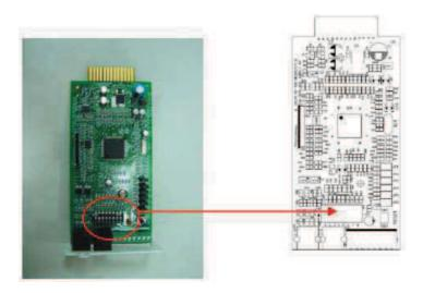
There are 8 DIP-switches that can be used to a set a "BIT matrix". The desired address must therefore be converted into a binary format.
