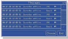
The Solar-Log<sup>™</sup> generates messages depending on configuration for errors and faults, or just to give
