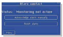
The SoleilLog<sup>1000</sup> constantly monitors its internal alarm contact. Once this has been interrupted the alarm is triggered. What happens here can be configured in the dialogue "Config/Advanced/Alarm contact" (notification by email/SMS/relay).
