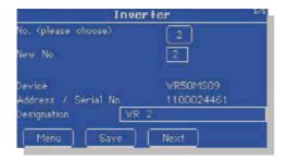
All dialogues relate always to a single inverter. Which inverter is currently being configured is shown in dialogue 1 above at "Number". This number can be changed by pressing on it. In this case a list of all inverters is displayed which you can select from.
