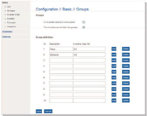
Up to 10 plant groups can be set, with up to 15 inverters per group. Via the Add and Remove buttons, you can easily assign individual inverters or remove them from a group. After saving the changes, the settings are immediately active.
