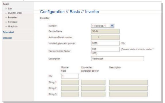
The inverters are always sorted by the serial number or communication address. If the order is to be changed, this can be changed through the dialogue "Inverter order". Please note that the ordering should be carried out immediately after inverter detection.
