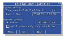
The time (clock) is important, which is already setup from the factory by default, but after prolonged storage can be lost. Then a random value is there, that has to be corrected.
