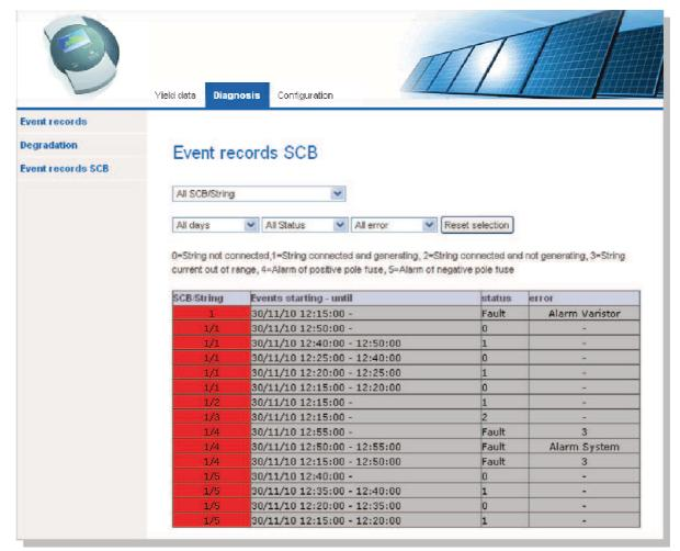
The selection functions can be used to filter data specifically for individual SCBs or by date in order to detect problems faster.
