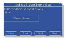
In dialogue 3, the RS485/422-B interface is defined, here you can also set the "Fronius" inverter.
