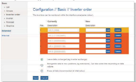
On the left side the inverters are listed in the old order, with the current position, the inverter name and serial number/address number. On the right side, the order can be changed by clicking on "Add".
