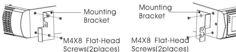
FIG.5 Installing the Mounting Brackets
