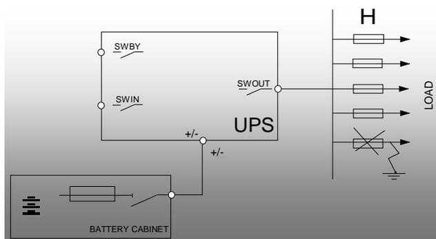
In order to select the correct protection devices to be inserted downstream of the SAFEPOWEREVO-HFT, the following two operating modes have to be taken into consideration: **mains power supply** and **battery power supply**.
