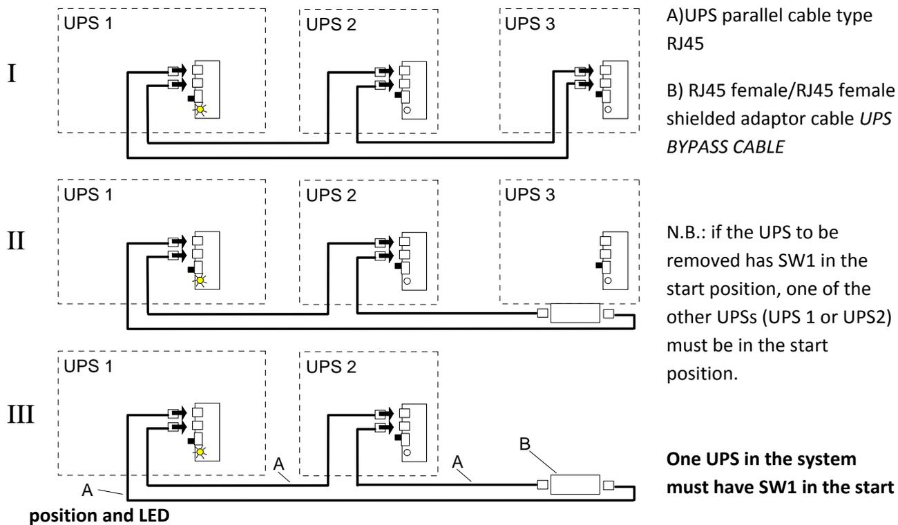
Phase I Shut down the UPS (3) that is to be removed. Remove the signal cables of the UPS to be removed.
