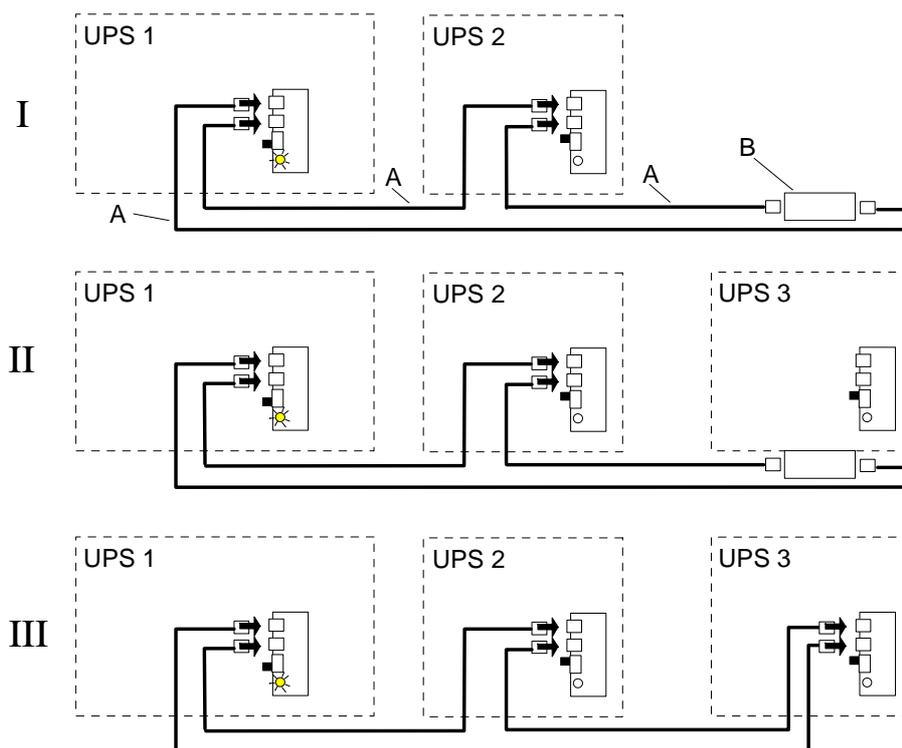
A) UPS parallel cable type RJ45
