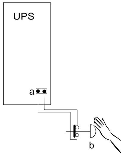
a - EPO terminal board located on the UPS
