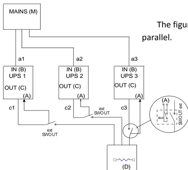
The figure shows an example of three units connected in parallel.
