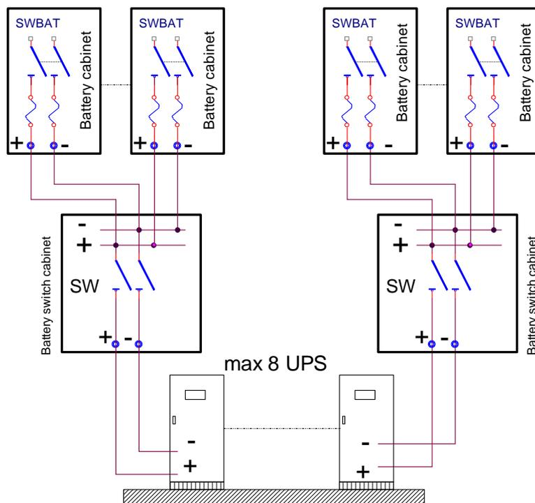
Several SAFEPOWEREVO-HFTs connected to the same battery
