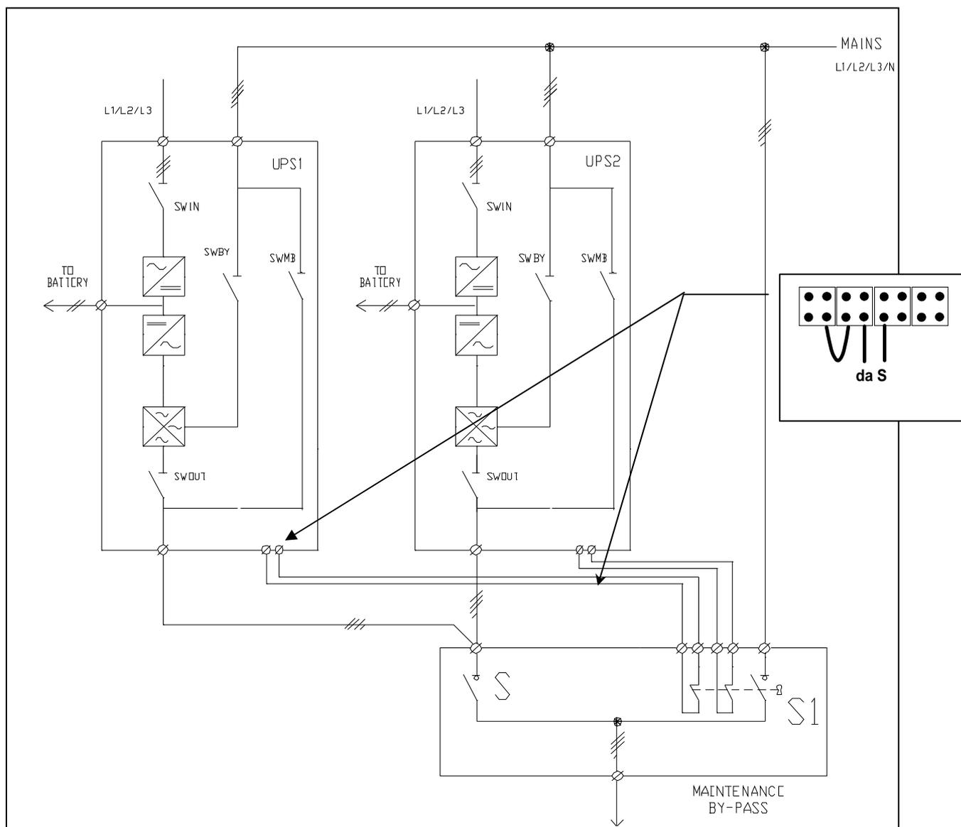
Mains, load and battery connections.
