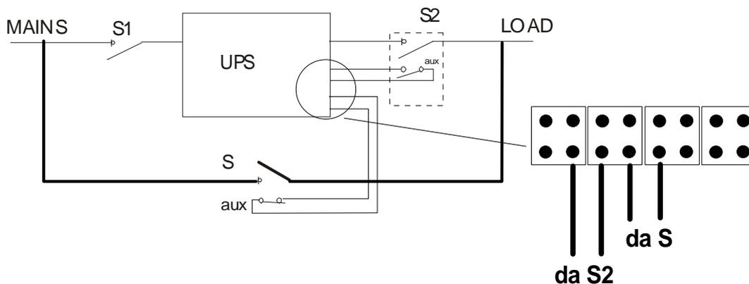
Additional output disconnector S2, additional disconnector S of the external maintenance by-pass.
